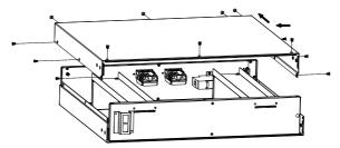
Step 5: Once the battery box is opened, remove the battery fixing plate present on the left side of the unit by unscrewing the 2 screws.
