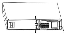
Step 4: Remove the metal top cover of the battery box by unscrewing 8 screws present on the two sides (4 on the right side and 4 on the left side), 3 screws on the top and 4 screws on the back side.
