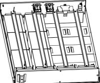
**Note:** To install the second branch of batteries, repeat the same procedure on the right side of battery box.
