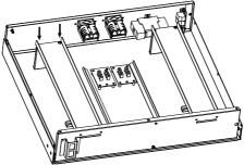
Pull up first and then push the battery fixing plate.
