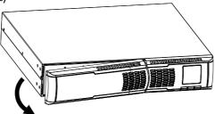
Step 3: Remove the fixed part of the front panel by removing 2 screw present.
