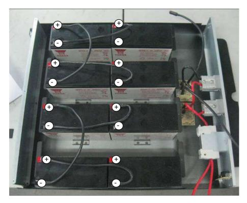
**Note:** The cable connection from external battery connector to PCB is already present inside the battery box. All the other cable connection should be followed by wiring diagram.
