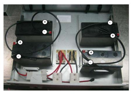
**Note:** The cable connection from external battery connector to PCB is already present inside the battery box. All the other cable connection should be followed by wiring diagram.
