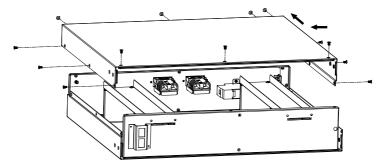
Step 5: Once battery box is opened, remove the battery fixing plate present on the left side by unscrewing 2 screws present.
